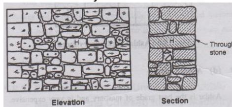
**4) Squared rubble masonry (uncoursed):** - Squared stone means whose edges have been made roughly straight. The stones are roughly dressed and are laid at random on their natural beds so that they are interlocked. The joints should not exceed 13 mm thickness. The gaps are filled by mortar and stone chips.
