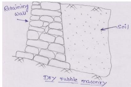
**2) Uncoursed rubble masonry:** - In uncoursed rubble masonry, stones or rubbles are used without any dressing. The mason select the stones at random from heap and lays them in line and plumb so as to form a strong bond.
