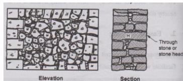
**3) Coursed rubble masonry:** - In this type of masonry, stones are placed to level course. Size of stones used are in between 50mm to 200mm. Joints are about 15mm in thickness.
