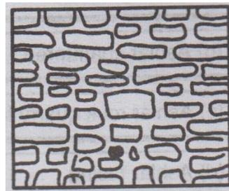
**5) Squared rubble masonry (coursed):** - In this type of masonry, semi-dressed stones are used. The stones are arranged in regular courses. Stones of equal height should be used in a course or two to three stones are kept above each other to make up the height of course. Mortar joint should not exceed 13 mm. the stone used in this masonry should be of uniform
