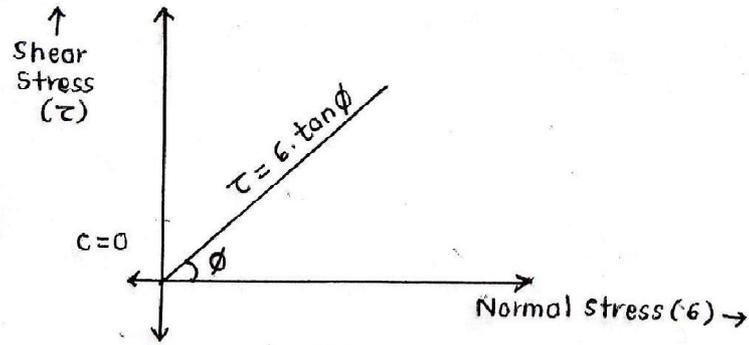
Fig.No. 4(b): Shear strength envelope for cohesionless soil
