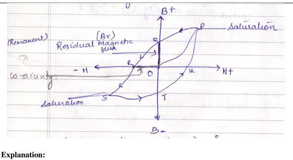
By plotting values of flux density, ( B ) against the field strength, ( H ) we can produce a set of **curves** called **Magnetization Curves**, Magnetic Hysteresis **Curves** or more commonly B-H **Curves**. The phenomenon of magnetization and demagnetization of ferromagnetic material is known as hysteresis.
